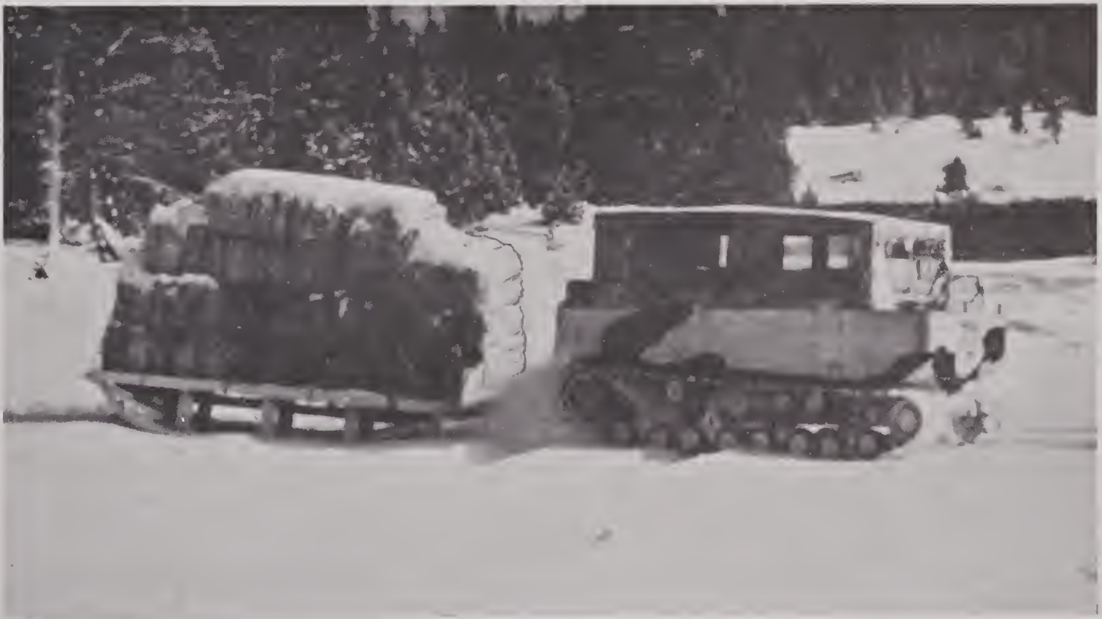
FIGURE 60. At Camp Hale, Colorado, M-29 Weasel (with trailer) serves for training and for transportation in winter.
